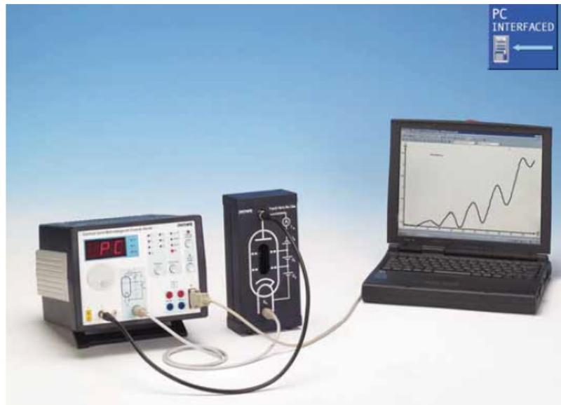
FIG. 2: The Franck-Hertz instrument captured from [2,4].
