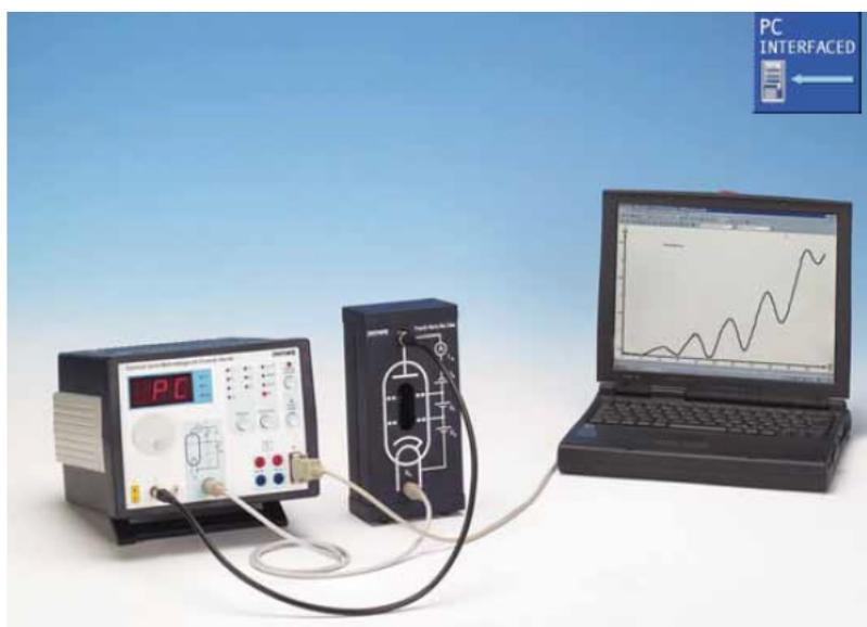
FIG. 2: The Franck-Hertz instrument captured from [2,4].
