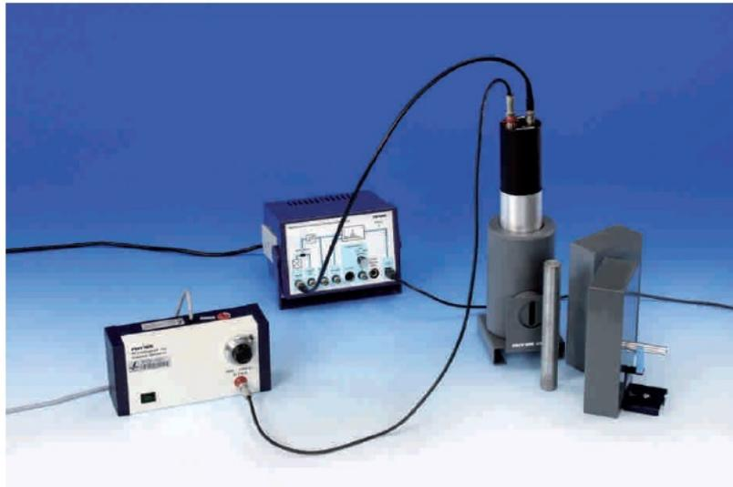
FIG. 2: The Compton effect *via* multichannel instrument[2,4]
