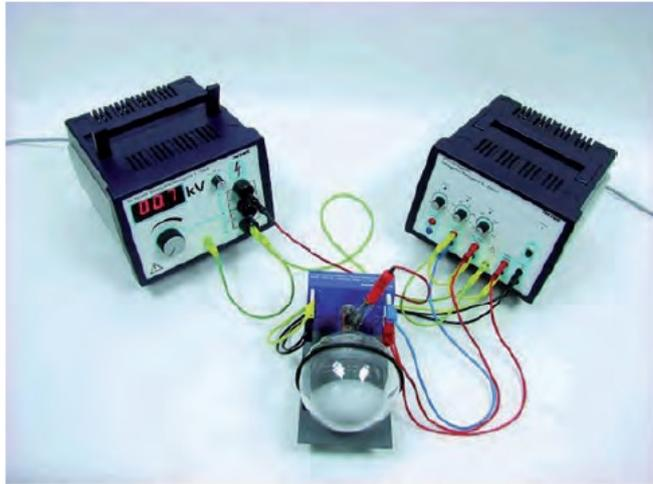
FIG. 1: The electron diffraction instrument captured from [2,4].
