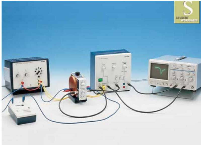
FIG. 1: The Electronic spin resonance instrument captured from [2,4].
