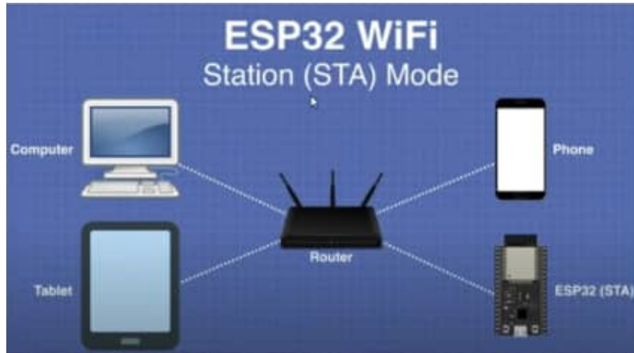
Figure 1.10: STA Mode in ESP32 Wireless Networking.
