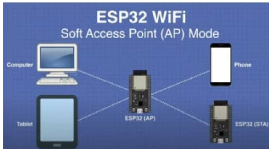
Figure 1.11: AP Mode in ESP32 Wireless Networking.
