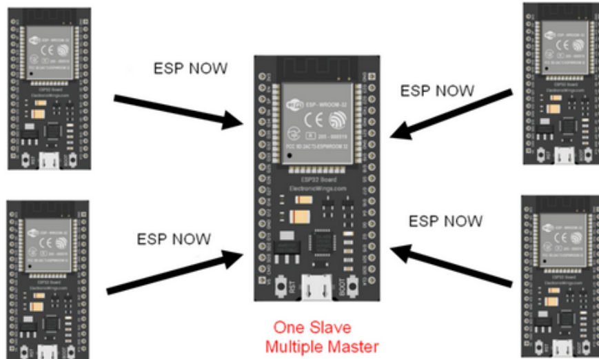
Figure 1.9: ESP-NOW Multiple-to-One Board Communication.
